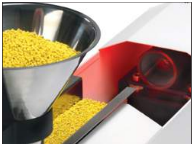
HAYER CPA 2-1 in the measurement of plastic granules
